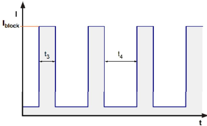
Anlaufstrom @ 48 V ( $I = 500\text{MA/div}$  ;  $t = 2\text{s/div}$ )
