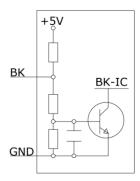
5.8 ALM: Alarm Output: When the circuit is in an alarm state, this port outputs 0V; when there is no alarm, it outputs 5V.
