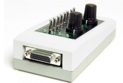
The 8 switches on the PA0160-24 for input signals can be activated either as a switch or as a push button depending whether they are activated to the left or the right. In the middle they are neutral.
