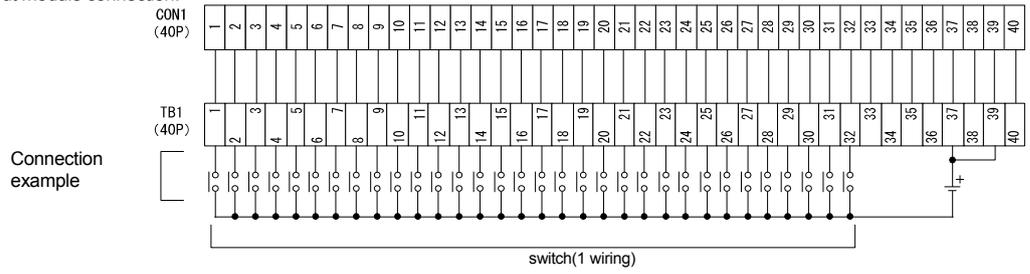
(2) When the negative common input module connection.
