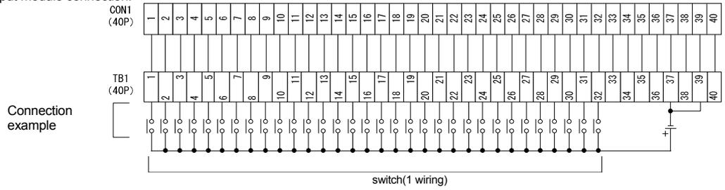
(3) When the sink output module connection.
