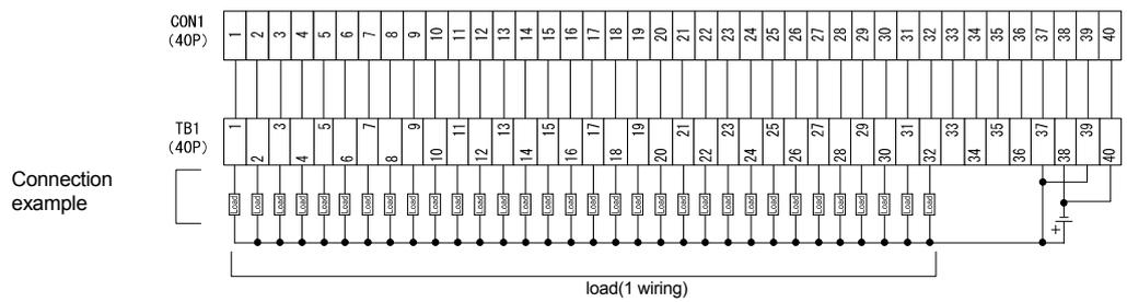
(4) When the source output module connection.
