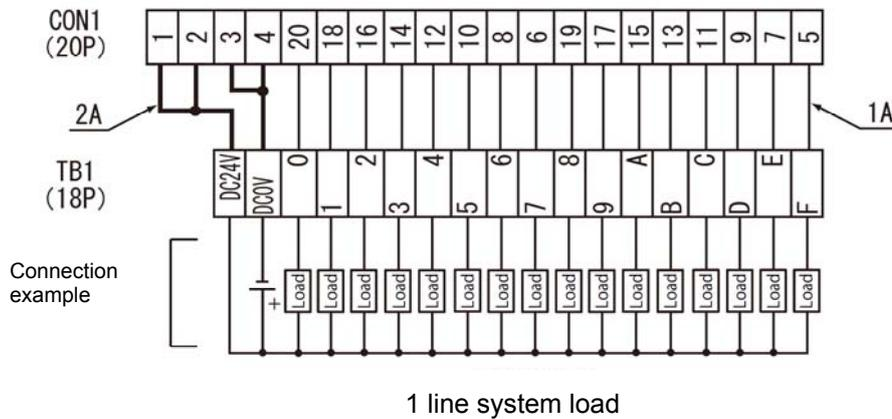
(4) When the source output module connection.
