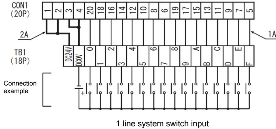
(3) When the sink output module connection.
