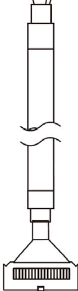
Insert the connector to the back, and then fully secure the connector with a clip.
