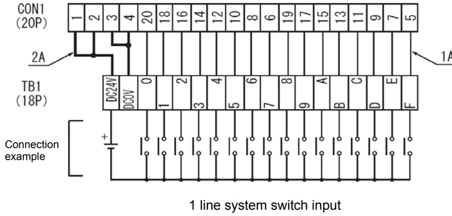
(2) When the negative common input module connection.
