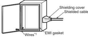
\*1 These wires are used to improve the conductivity between the door and control cabinet.
